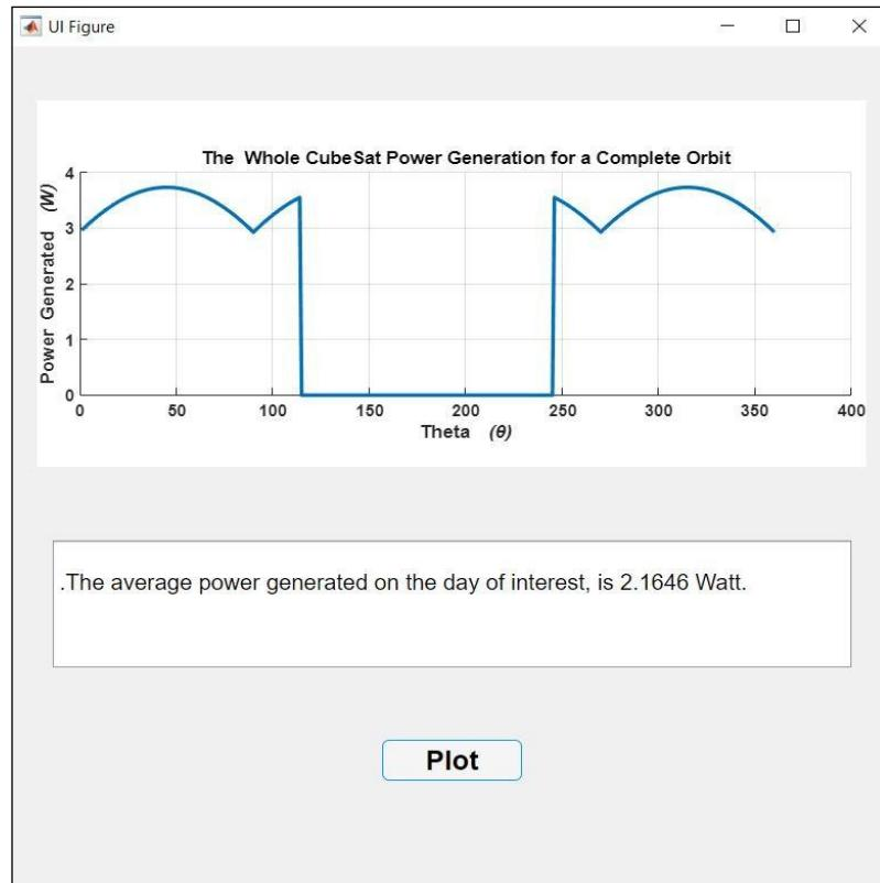
This result tab illustrates the total power generated by the CubeSat in one complete orbit. The source of power generation on the CubeSat is solar panels. In our simulation, we have assumed to have a solar panel on each surface.
