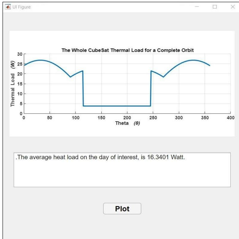
This tab generates result for the full thermal load of the whole CubeSat for one complete orbit. The total thermal load result is inclusive of total direct solar load, total albedo load and total infra-red load that was measured on each surface.
